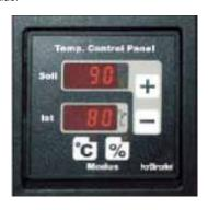
the actual water temperature is measured at the heating coil outlet and displayed in °C. The temperature can be raised by increasing the percentage of time that the burner is operating, or lowered by reducing the percentage.
