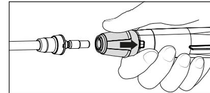
5. First pull back the retaining sleeve of the safety trigger gun, then insert lance into the plug coupling sconnection of the safety trigger gun.
