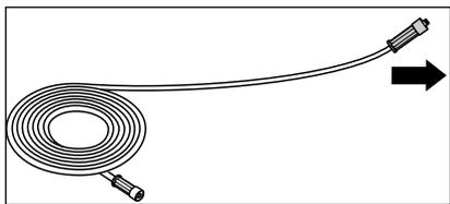
2. Unwind high pressure hose straight and without nooses. When using high pressure hose extensions take care that the max. length of 20 m is not exceeded!
