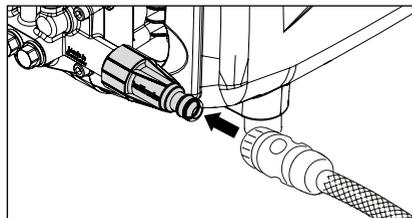
**8.** Connect the water hose to water inlet sieve (minimum requirements; 5 m hose length, cross-section 3/4", 10 bar). The high pressure cleaner may be connected to a water mains (1-10 bar pre-pressure) with either cold or hot water (up to 60 °C).
