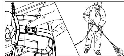
**10.** Switch on high pressure cleaner with opened safety trigger gun. Bleeding of the high pressure cleaner: Pull and release trigger of safety trigger gun several times. Start cleaning task.
