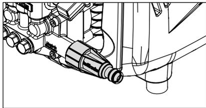
**7. Check water inlet filter for cleanliness prior to putting the high pressure cleaner into operation.**
