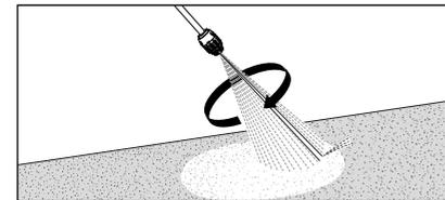
**11.** When using the filth killer lance make sure that lance points downward when starting.
