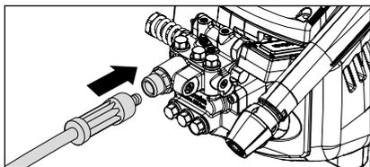
3. Plug screw high-pressure hose included in scope of delivery at pump outlet and tightly screw pressure-tight.
