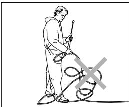
Never pull the high pressure hose if it has formed kinks or "nooses"! Never pull the high pressure hose over sharp edges!
