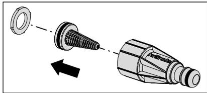
**7.1** If contaminated, remove the filter and thoroughly rinse it with clear water and clean it with the other parts.
