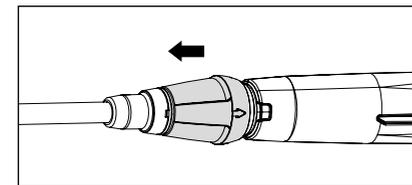
6. After insertion of the lance, release retaining sleeve and make sure that the lance is in a secure position.
