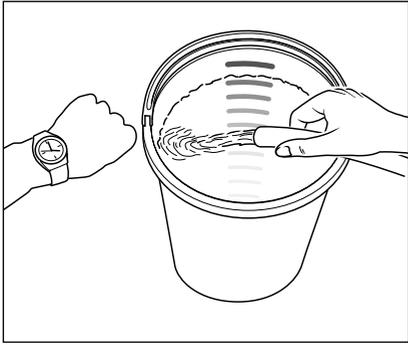
Lack of water occurs more often than you probably believe. The more powerful a high pressure cleaner is the greater is the danger that a lack of water occurs. If there is only an insufficient amount of water available, cavitation (water-gas mixture) arises inside the high pressure pump, which is normally noticed too late or even not at all. **The high pressure pump will be destroyed.** Please check the available quantity of water by filling a bucket with liter scale for one minute.
