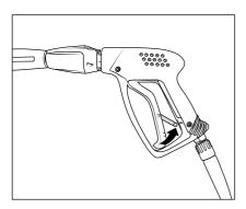
Apply the safety catch on the safety trigger gun after each use in order to prevent unintentional spraying!
