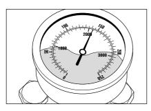
Having closed the trigger gun with safety catch, the high pressure cleaner must shut down and the stainless steel pressure gauge must show "0" bar. If not shut down and the stainless steel pressure gauge continuously shows full pressure, this could be due to leakage at the high pressure pump, at the pressure switch, at the high pressure hose or at the trigger gun with safety catch.
