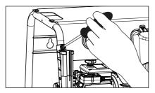
Attach the holder for the lances with a screwdriver and the enclosed screws.
