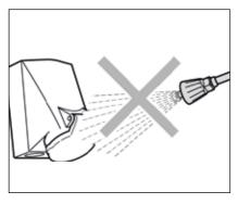
Never direct the high pressure jet at power sockets or any other electrical installations!
