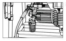
**3.** Tightly screw together high pressure hose and safety trigger gun.
