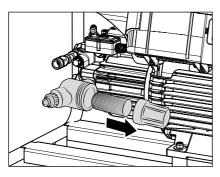
10. If using a water inlet filter check it for cleanliness prior to each startup.
