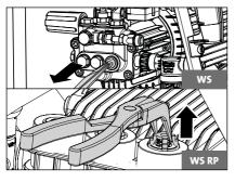
Take out valve body and O-ring by means of needle nose pliers. Check O-ring for damage. In case of a damage the O-ring has to be replaced.
