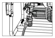
11. Connect the water hose to water inlet sieve. The high pressure cleaner may be connected to a water mains (1-10 bar pre-pressure) with either cold or hot water (up to 60 °C). The WS series provides the opportunity of sucking in water out of a container (see direct suction).
