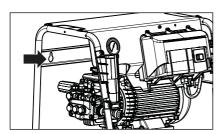
Please find the eyelets for wall mounting on the back of the device.
