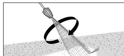
10. When using the turbokiller lance (optional) make sure that lance points downward when starting.
