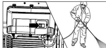
9. Switch on high pressure cleaner with opened safety trigger gun. Bleeding of the high pressure cleaner: Pull and release trigger of safety trigger gun several times. Start cleaning task.
