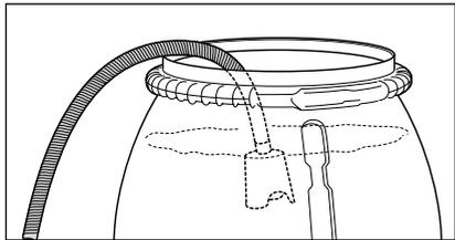
2. Put filled suction hose into the water-filled container and start the cleaning job.
