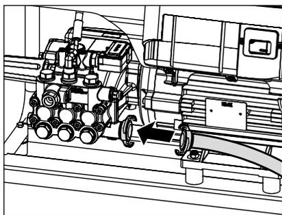
6. Connect water hose to water inlet (minimum requirements; 5 m hose length, cross-section ¾", 10 bar). The high pressure cleaner may be connected to a water mains (1-10 bar pre-pressure) with either cold or hot water (up to 60 °C). The WS-RP/WSC-RP-series provides the opportunity of sucking in water out of a container (see direct suction).
