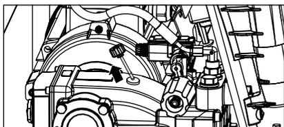
7. The oil level must reach to the upper edge of the mark.
