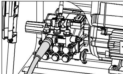
2. Plug screw high-pressure hose included in scope of delivery at pump outlet and tightly screw pressure-tight.
