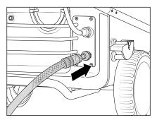
11. Connect water hose to water inlet (minimum requirements; 5 m hose length, cross-section ¾", 10 bar). The highpressure cleaner may be connected to a water mains (1-10 bar pre-pressure) with either cold or hot water (up to 60 °C). The therm-1-series provides the opportunity of sucking in water out of a container (see direct suction).
