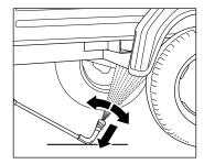
Always pay attention to the underbody lance resting on the surface! Bear in mind when using a curved or angled spraying lance that there is a significant amount of torque in the recoil! (The underbody lance is available as optional accessory).
