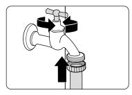
**Step 2:** Connect water hose to water inlet. Open water tap.
