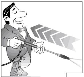
The recoil is less than 20 Nm.
