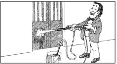
Blasting old paint, rust and facades: sandblasting injector with suction lance and 3 m PVC-hose and ST 30 nipple M 22 x 1,5
