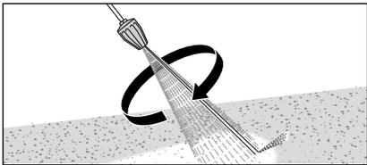
14. When using the turbokiller lance make sure that lance points downward when starting.
