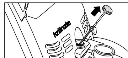
11. **Each time check oil level at the oil dipstick prior to putting the high pressure cleaner into operation.**
