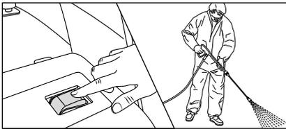
13. Switch on high-pressure cleaner with opened safety trigger gun. Bleeding of the high-pressure cleaner: Pull and release trigger of safety trigger gun several times. Start cleaning task.
