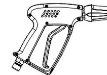
2. Safety trigger gun with plug coupling
