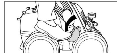
2. For moving the high-pressure cleaner to the place of use, please release locking break.
