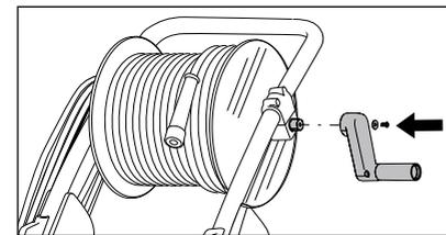
1. For high-pressure cleaners with hose drum the enclosed hand crank must be applied prior to first operation. Plug the hand crank onto the hexagon and attach it with the enclosed screw and washer.
