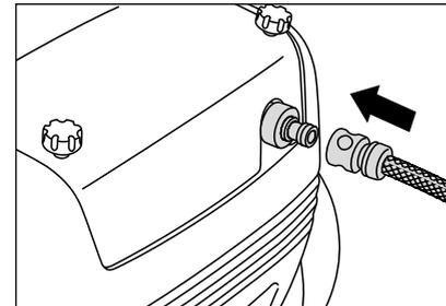
10. Connect water hose to water inlet (minimum requirements; 5 m hose length, cross-section 3/4", 10 bar). The high pressure cleaner may be connected to a water mains (1-10 bar pre-pressure) with either cold or hot water (up to 60 °C). The large quadro series provides the opportunity of sucking in water out of a container (see direct suction).
