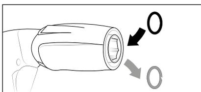
Switch off the cleaner. Shortly press the trigger of the trigger gun with safety catch to decrease the pressure. Remove high-pressure hose, trigger gun with safety catch and lance and check the O-rings. If the O-rings are damaged they have to be replaced.
