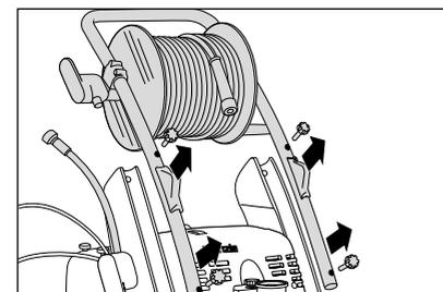
4. For transport purposes the handle can be taken off easily. First detach the high-pressure hose from the hose drum. After that, unscrew the fixing screws and detach handle and hose drum
