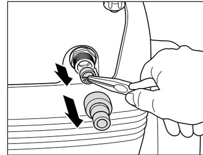
9. **Check water inlet filter for cleanliness prior to putting the high-pressure cleaner into operation.**
