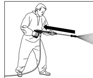
When using high-pressure water for cleaning, make sure that there is a clearly noticeable recoil effect on the lance. Therefore ensure a firm footing (see technical data).
