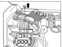
Remove the large right hood from the high-pressure cleaner and release the oil drain hose from the inside of the device. It is connected to the oil drain screw. Then open the red oil filling plug at the top of the silver oil housing and then the closure cap at the end of the hose. The oil is to be caught in the reservoir and disposed of in an approved manner. Close the end of the hose. Only then top up fresh oil.
