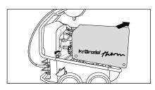
**12.** For getting access to the interior fitting of the high-pressure cleaner, loosen screws at the cover. Remove cap carefully.
