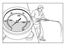
The stainless steel pressure gauge shows low pressure despite fully turned up pressure regulation. The water from the lance comes in squirts. The high-pressure hose vibrates.
