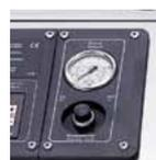
Large stainless steel pressure gauge and switch for detergent pump
