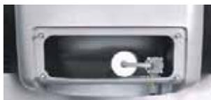
Integrated water buffer tank with float valve to prevent against any irregularities in the water supply. This reduces the risk of cavitation occurring in the pump - which is a major cause of high pressure pump failure.
