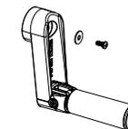
8. Crank handle with fastening screw
