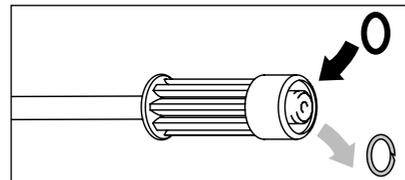
Switch off the high pressure cleaner. Shortly press the trigger of the safety trigger gun to decrease the high pressure cleaner. Unscrew high pressure hose, safety trigger gun and lance and check the O-rings. If the O-rings are damaged they have to be replaced.
