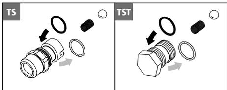
If sealing rings are defective replace O-rings at once.
