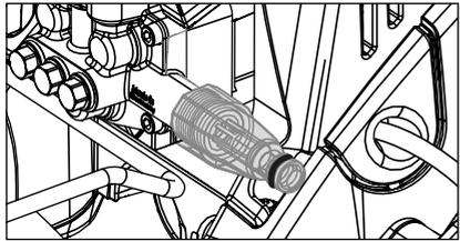
**9. Check water inlet filter for cleanliness prior to putting the high pressure cleaner into operation.**
