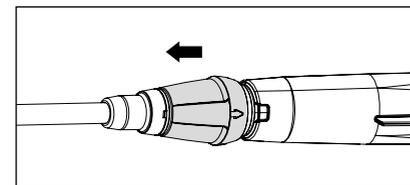
8. After insertion of the lance, release retaining sleeve and make sure that the lance is in a secure position.
