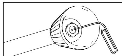
If the problem still exists, take wire (paper clip) and push through nozzle opening. If this procedure is not successful, the nozzle has to be replaced.
