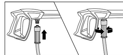
6. Tightly screw together high pressure hose and safety trigger gun.
