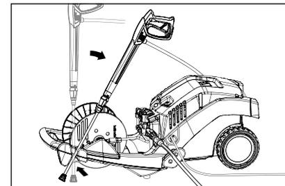
**14.** The K 1050 TS/TST units are equipped with a support for the safety trigger gun with lance during breaks.
