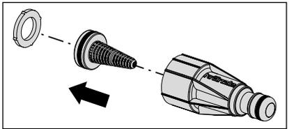
**9.1** If contaminated, remove the filter and thoroughly rinse it with clear water and clean it with the other parts.
