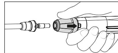
7. First pull back the retaining sleeve of the safety trigger gun, then insert lance into the plug coupling connection of the safety trigger gun.
