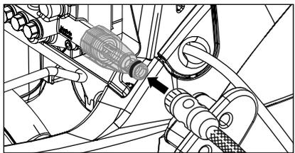
**10.** Connect the water hose to water inlet sieve (minimum requirements; 5 m hose length, cross-section 3/4", 10 bar). The high pressure cleaner may be connected to a water mains (1-10 bar pre-pressure) with either cold or hot water (up to 60 °C).
