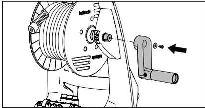
2. For high pressure cleaners with hose drum the enclosed hand crank must be applied prior to first operation. Please set up the high pressure cleaner. Plug the hand crank on to the hexagon and attach it with the enclosed screw and washer.
