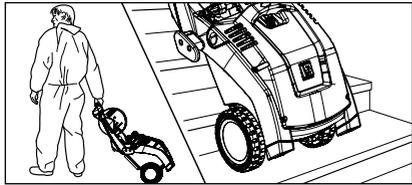
3. Move high pressure cleaner to the job site. The K 1050 TS/TST is a movable high pressure cleaner with sturdy trolleys ideally suited for difficult terrain and stairs.
