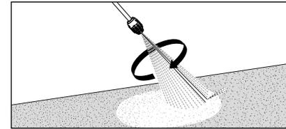
**13.** When using the filth killer lance make sure that lance points downward when starting.
