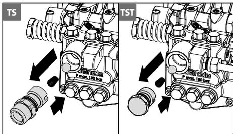
Remove check body and check O-Ring for soiling or damage. Also check seal seat inside pump housing for soiling or damage.
