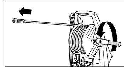
5. For high pressure cleaners with hose drum, however, it must be uncoiled completely. For high pressure cleaners without hose drum the high pressure hose included in the scope of the delivery must be screwed with the pump outlet in a tight and pressure tight manner. Unwind high pressure hose straight and without nooses.
