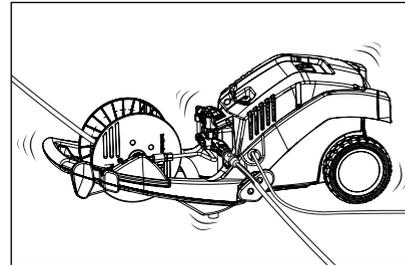
Having closed the safety trigger gun, the high pressure cleaner must shut down. Failure to shut down may be caused by leakage in the high pressure pump, the switch, the high pressure hose, the safety trigger gun or the lance.
