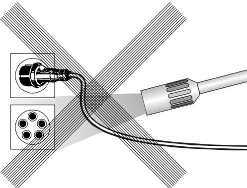
**Never direct the water jet at a power socket !**
