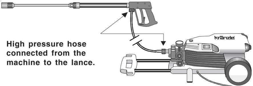
**High pressure hose connected from the machine to the lance.**
