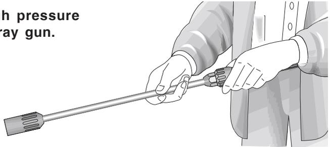
3. Unwind the high pressure hose without leaving kinks or "nooses" and connect it to the spray gun and pump. When using extension hoses, use max. 20 m high pressure hose, or 2 x 10 m with hose connectors.
