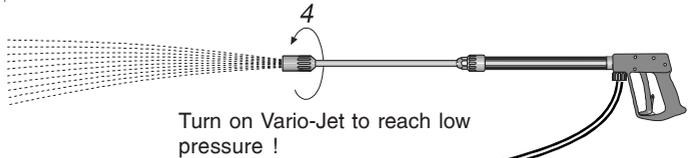
A mixing ratio of 3-5% is achieved when the Vario-Jet is fully turned on. pH value neutral 7-9.
