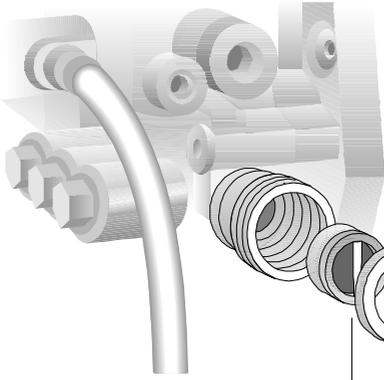
4. The machine can be connected to a pressurised water line with cold or 60°C hot water (see page 2).
