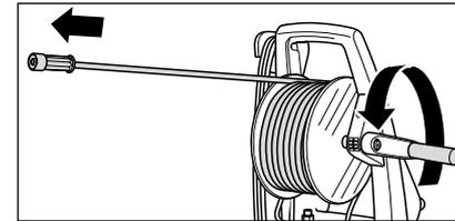
4. For high-pressure cleaners with hose drum, however, it must be uncoiled completely. For high-pressure cleaners without hose drum the high-pressure hose included in the scope of the delivery must be screwed with the pump outlet in a tight and pressure tight manner. Unwind high-pressure hose straight and without nooses. The high-pressure hose may leave signs of abrasion on some floors. Alternatively, please also find non-marking high-pressure hoses in our range.
