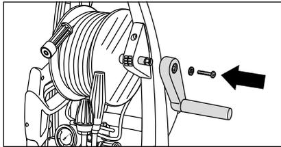
2. For high-pressure cleaners with hose drum the enclosed hand crank must be applied prior to first operation. For this purpose, please set up the high-pressure cleaner. Plug the hand crank onto the hexagon and attach it with the enclosed screw and washer.
