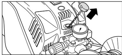
**10. Each time check oil level at the oil dipstick prior to putting the high pressure cleaner into operation. (Take care that cleaner is in horizontal position!) Oil level must reach until the upper edge of marking "OK".**
