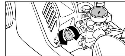
**14. Adjust operating pressure infinitely using the rotary handle. The maximum pressure is factory-set.**
