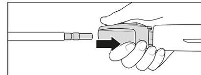
6. First pull back the retaining sleeve of the safety trigger gun, then insert lance into the plug coupling sconnection of the safety trigger gun.
