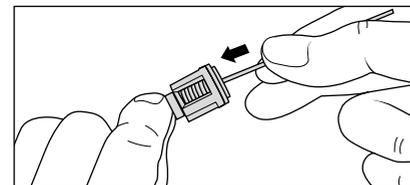
Do not forget the O-ring during reassembly!
