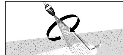
**13. When using the dirtkiller lance make sure that lance points downward when starting.**
