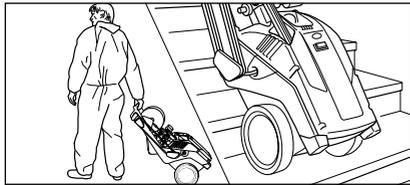
3. Move high-pressure cleaner to the job site. The K 1152-series is a movable high-pressure cleaner with sturdy trolleys ideally suited for difficult terrain and stairs.
