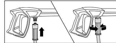
5. Mount the grey rotating screw connection of the high-pressure hose onto the trigger gun incorporating a safety catch. Afterwards screw together ensuring a snug and pressure-tight fit.
