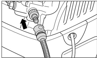
**9. Connect water hose to water inlet (minimum requirements; 5 m hose length, cross-section 3/4", 10 bar). The high-pressure cleaner may be connected to a water mains (1-10 bar pre-pressure) with either cold or hot water (up to 60 °C).**
