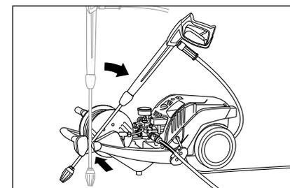
**15. The K 1152-series units are equipped with a support for the safety trigger gun with lance during breaks.**
