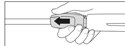
7. After insertion of the lance, release retaining sleeve and make sure that the lance is in a secure position.
