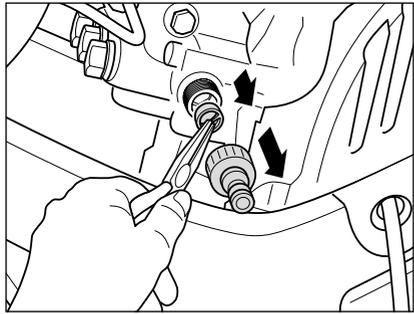
**8. Check water inlet filter for cleanliness prior to putting the high-pressure cleaner into operation.**
