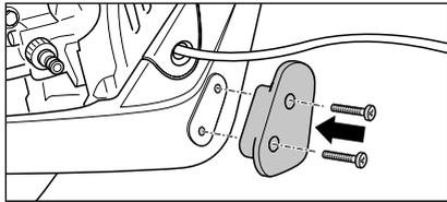
1. Use the supplied screws to fasten the lower cable retractor of the power supply cable in the place provided on the frame.
