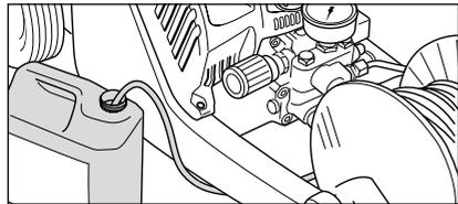
1. Place chemicals filter into container with additives
