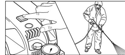
**12. Switch on high-pressure cleaner with opened safety trigger gun. Bleeding of the high-pressure cleaner: Pull and release trigger of safety trigger gun several times. Start cleaning task.**
