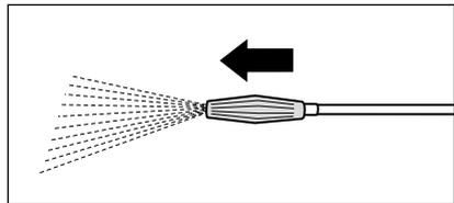
2. To reach the low pressure push Vario nozzle to the front so that the injector can suck in the additives.
