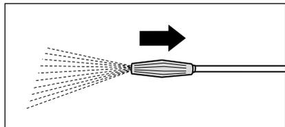
3. When pushing the Vario nozzle backwards, chemicals supply is automatically stopped, high-pressure cleaner changes in high-pressure mode. Let additives take effect and then spray off with high-pressure.
