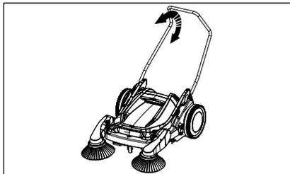
2. The push bar can be set to the desired working height. This is easier on your back.
