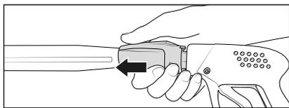
**! The plug coupling must not be actuated/handled during operation! High risk of injury!**
