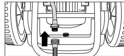
2. Screw suction hose with suction filter (Item.-no.: 150383) with connecting hose using a spreaded steel pipe fitting (Item.-no.: 46004).
