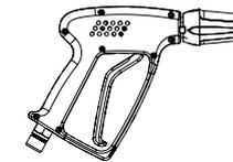
2. Safety trigger gun with plug coupling
