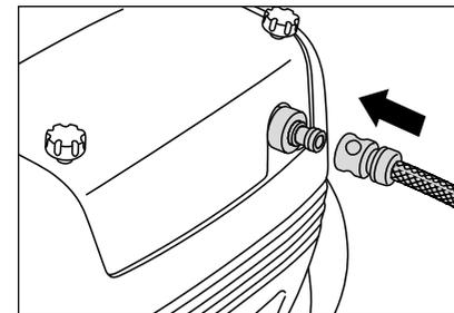
10. Connect water hose to water inlet (minimum requirements; 5 m hose length, cross-section 3/4", 10 bar). The high pressure cleaner may be connected to a water mains (1-10 bar pre-pressure) with either cold or hot water (up to 60 °C). The large quadro series provides the opportunity of sucking in water out of a container (see direct suction).
