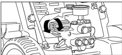
15. Adjust operating pressure infinitely using the rotary handle. The maximum pressure is factory-set.
