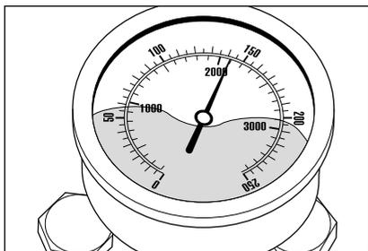
Having closed the trigger gun with safety catch, the high-pressure cleaner must shut down and the stainless steel pressure gauge must show „0“ bar. If not shut down and the stainless steel pressure gauge continuously shows full pressure, this could be due to leakage at the high-pressure pump, at the pressure switch, at the high-pressure hose or at the trigger gun with safety catch.
