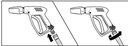
7. First pull back the retaining sleeve of the safety trigger gun, then insert lance into the plug coupling connection of the safety trigger gun.
