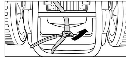
1. Unscrew connecting hose between high-pressure pump and water tank.
