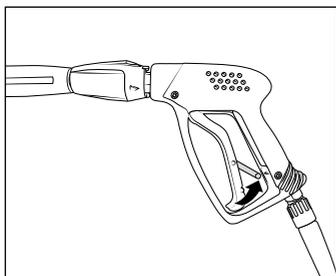
Apply the safety catch on the safety trigger gun after each use in order to prevent unintentional spraying!
