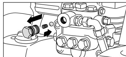
Remove check body and check O-Ring for soiling or damage. Also check seal seat inside pump housing for soiling or damage.
