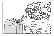
Place chemicals filter into container with additives
