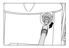
8. Connect water hose to water inlet (minimum requirements; 5 m hose length, cross-section ¾", 10 bar). The high-pressure cleaner may be connected to a water mains (1-10 bar pre-pressure) with either cold or hot water (up to 60 °C). The medium quadro series provides the opportunity of sucking in water out of a container (see direct suction).
