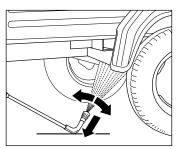
Always pay attention to the underbody lance resting on the surface! Bear in mind when using a curved or angled spraying lance that there is a significant amount of torque in the recoil!
