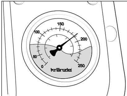
Having closed the trigger gun with safety catch, the high-pressure cleaner must shut down and the stainless steel pressure gauge must show the permitted deactivation pressure (see rating plate). If not shut down and the stainless steel pressure gauge continuously shows full pressure (device does not switch to bypass), this could be due to leakage at the high-pressure pump, at the pressure switch, at the high-pressure hose or at the trigger gun with safety catch.
