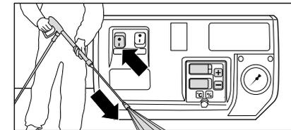
2. Switch on high-pressure cleaner with opened trigger gun (trigger pulled). Bleeding of the high-pressure cleaner: Pull and release trigger of trigger gun with safety catch several times. Start with cleaning process.
