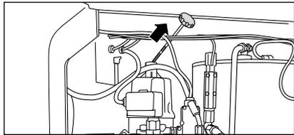
13. **Each time check oil level at the oil dipstick prior to putting the high-pressure cleaner into operation.** Oil level must reach until the upper edge of marking "OK". See chapter „Care and Maintenance“ in these operating manual.
