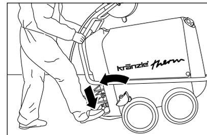
5. The therm-1-series is a movable high-pressure cleaner with sturdy trolleys ideally suited for difficult terrain. For steering the high-pressure cleaner put the foot against the tipping support and then pull the device towards you.
