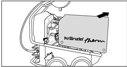
12. For getting access to the interior fitting of the high-pressure cleaner, loosen screws at the cover. Remove cap carefully.
