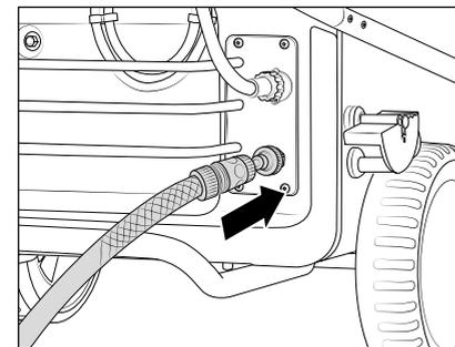
11. Connect water hose to water inlet (minimum requirements; 5 m hose length, cross-section 3/4", 10 bar). The high-pressure cleaner may be connected to a water mains (1-10 bar pre-pressure) with either cold or hot water (up to 60 °C). The therm-1-series provides the opportunity of sucking in water out of a container (see direct suction).
