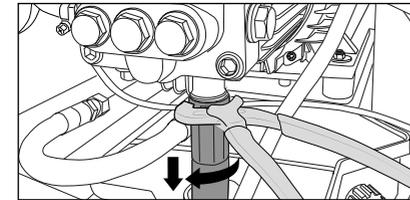
1. Unscrew connecting hose between high-pressure pump and water tank.
