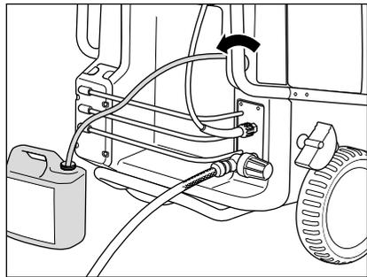
1. Place chemicals filter into container with additives.
