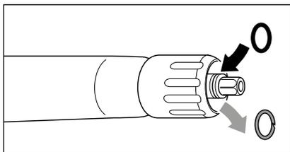
Switch off the cleaner. Shortly press the trigger of the trigger gun with safety catch to decrease the pressure. Remove high-pressure hose, trigger gun with safety catch and lance and check the O-rings. If the O-rings are damaged they have to be replaced.
