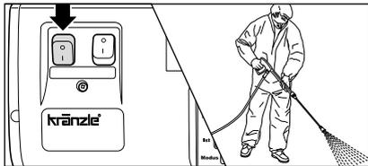
2. Switch on high-pressure cleaner with opened trigger gun (trigger pulled). Bleeding of the high-pressure cleaner: Pull and release trigger of trigger gun with safety catch several times.
