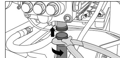
2. Screw suction hose with suction filter (Item.-no.: 150383) with connecting hose using a spreaded steel pipe fitting (Item.-no.: 46004).
