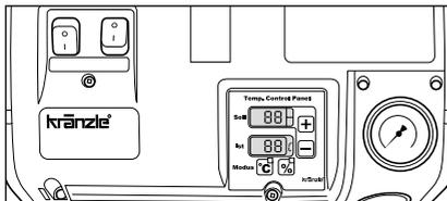
3. Set desired temperature at the thermostat. (Min. temperature 40 °C). On the subject of thermostat settings, see chapter "Functional details" in these operating manual.
