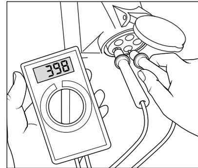
If there are too many collectors in your proximity connected to the network at the same time, the available voltage and the current intensity may decline. Consequently the motor of the high-pressure cleaner does not start or even blows. The power supply cable may also be insufficient if the power supply cable is too long or too thin. If extension cables are too long, this may lead to a voltage drop causing malfunctions or start-up difficulties.
