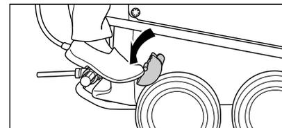
4. For moving the high-pressure cleaner to the place of use, please release locking break. The high-pressure cleaner **must not be** pulled with connected water supply hose!
