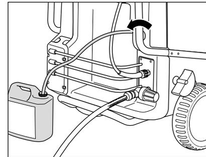
1. Place chemicals filter into container with additives.
