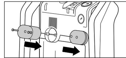
1. Install the mains cable holders with the screws.
