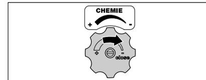
3. By closing the detergent valve the supply of detergent is stopped.
