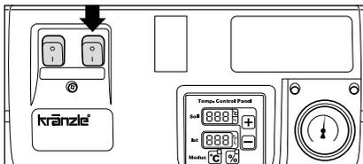
4. Switch on heater switch. The water is heated up and constantly kept at the set temperature.
