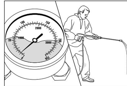
The stainless steel pressure gauge shows low pressure despite fully turned up pressure regulation. The water from the lance comes in squirts. The high-pressure hose vibrates.
