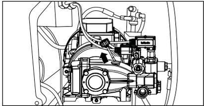
13. **Each time check oil level at the oil dipstick prior to putting the high-pressure cleaner into operation.**
