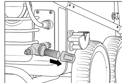
10. Check water inlet filter for cleanliness prior to putting the high-pressure cleaner into operation.
