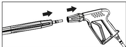
9. After insertion of the lance, release retaining sleeve and make sure that the lance is in a secure position. **Grease quick release nipple regularly using acid-free grease.**
