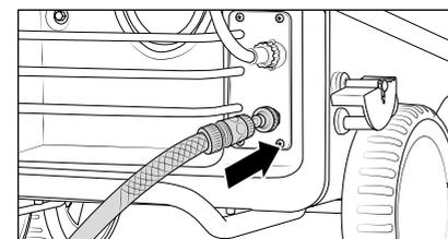
11. Connect water hose to water inlet (minimum requirements; 5 m hose length, cross-section 3/4", 10 bar). The high-pressure cleaner may be connected to a water mains (1-10 bar pre-pressure) with either cold or hot water (up to 60 °C).
