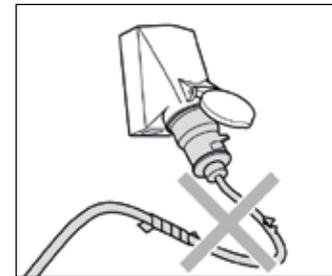
Only use a power supply cable in perfect working order! Do not damage or improperly repair the power cable (tearing, squeezing, running over, ...).
