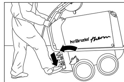
5. The therm-RP-series is a movable high-pressure cleaner with sturdy trolleys ideally suited for difficult terrain. For steering the high-pressure cleaner put the foot against the tipping support and then pull the device towards you.
