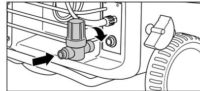
2. Install the water inlet filter (available as an option) at the water inlet.
