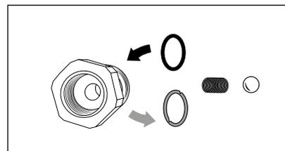
If sealing rings are defective replace O-rings at once.
