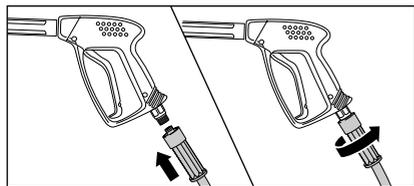
8. First pull back the retaining sleeve of the safety trigger gun, then insert lance into the plug coupling connection of the safety trigger gun.
