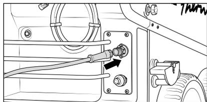
7. Tightly screw together high-pressure hose and safety trigger gun.
