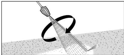
15. When using the turbokiller (available optionally), ensure that the lance is pointing down for start-up.
