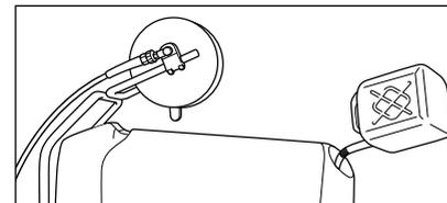
3. Prior to putting into operation fill fuel oil into the fuel tank. (fuel oil EL DIN 51 603 or diesel fuel DIN EN 590). Filling quantity 25 liters.
