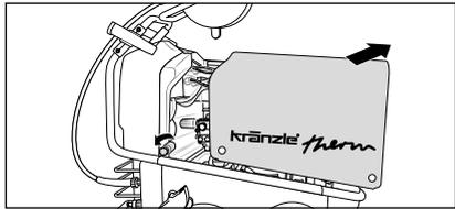
12. For getting access to the interior fitting of the high-pressure cleaner, loosen screws at the cover. Remove cap carefully.
