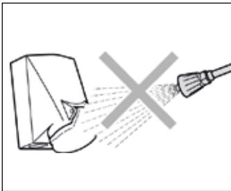
Never direct the high-pressure jet at power sockets or any other electrical installations! Within the working area, all live parts are to be protected from both water jet and spray mist.
