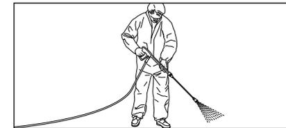
3. When starting the cleaning process do **not** aim the water jet towards the object you want to clean for at least 30 seconds. Maybe the water inside the combustion chamber has changed colour due to the rest time.
