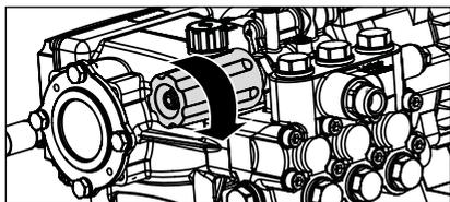
16. Adjust operating pressure infinitely using the rotary handle. The maximum pressure is factory-set.
