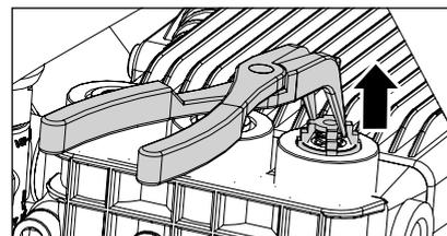
Take out valve body and O-ring by means of needle nose pliers. Check O-ring for damage. In case of a damage the O-ring has to be replaced.
