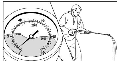
The stainless steel pressure gauge shows low pressure despite fully turned up pressure regulation. The water from the lance comes in squirts. The high pressure hose vibrates. (Inside the stainless steel pressure gauge is no water but a filling with glycerin to damp the vibration of the pointer.)
