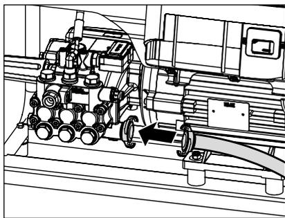
6. Connect water hose to water inlet (minimum requirements; 5 m hose length, cross-section 3/4", 10 bar). The high pressure cleaner may be connected to a water mains (1-10 bar pre-pressure) with either cold or hot water (up to 60 °C). The WS-RP/WSC-RP-series provides the opportunity of sucking in water out of a container (see direct suction).
