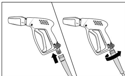
3. Mount the grey rotating screw connection of the high-pressure hose onto the trigger gun incorporating a safety catch. Afterwards screw together ensuring a snug and pressure-tight fit.
