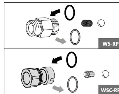
If sealing rings are defective replace O-rings at once.
