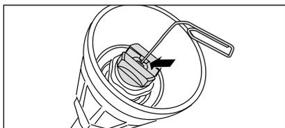
If the problem still exists, take wire (paper clip) and push through nozzle opening. If this procedure is not successful, the nozzle has to be replaced.
