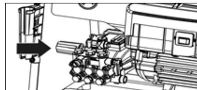
11. Adjust operating pressure infinitely using the rotary handle. The maximum pressure is factory-set.
