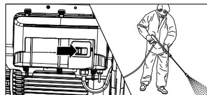
9. Switch on high pressure cleaner with opened safety trigger gun. Bleeding of the high pressure cleaner: Pull and release trigger of safety trigger gun several times. Start cleaning task.
