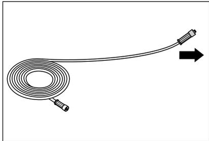
1. Unwind high pressure hose straight and without nooses. (When using high pressure hose extensions take care that the max. length of 20 m is not exceeded!)
