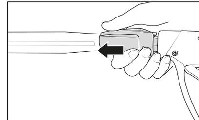
5. After insertion of the lance, release retaining sleeve and make sure that the lance is in a secure position.
