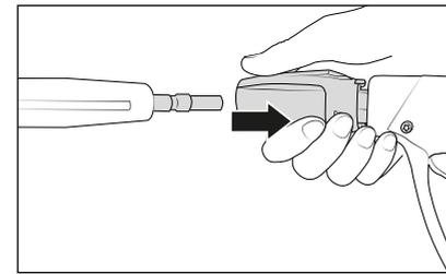
4. First pull back the retaining sleeve of the safety trigger gun, then insert lance into the plug coupling sconnection of the safety trigger gun.
