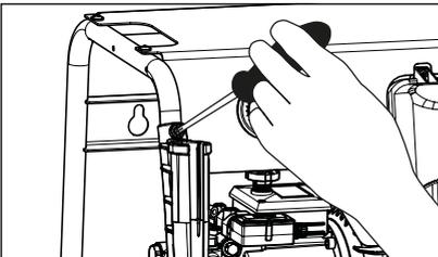
Attach the holder for the lances with a screwdriver and the enclosed screws.
