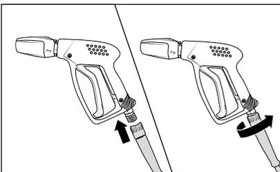
3. Tightly screw together high pressure hose and safety trigger gun.
