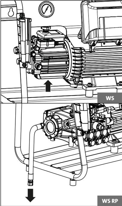
The first oil change should be carried out after approximately **50 operating hours**, then every year or after 250 operating hours. If the oil turns grey or white, you must change the oil. In case of exchanging oil being required, the oil drain screw must be opened above a container and the high pressure cleaner be emptied. The oil is to be caught in the reservoir and disposed of in an approved manner.
