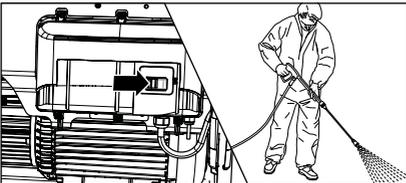
14. Switch on high pressure cleaner with opened safety trigger gun. Bleeding of the high pressure cleaner: Pull and release trigger of safety trigger gun several times. Start cleaning task.
