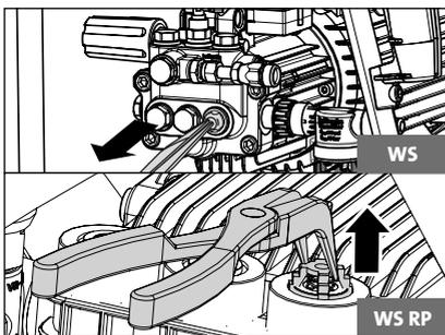
Take out valve body and O-ring by means of needle nose pliers. Check O-ring for damage. In case of a damage the O-ring has to be replaced.
