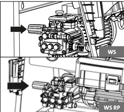
16. Adjust operating pressure infinitely using the rotary handle. The maximum pressure is factory-set.
