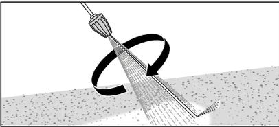
15. When using the turbokiller lance (optional) make sure that lance points downward when starting.
