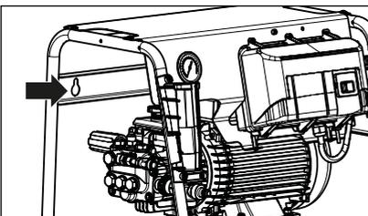
Please find the eyelets for wall mounting on the back of the device.
