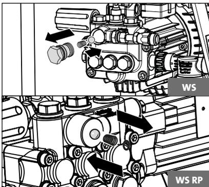
Remove check body and check O-Ring for soiling or damage. Also check seal seat inside pump housing for soiling or damage.
