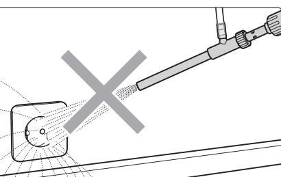
Do not point water and/or sandblast jet at any wall sockets!
