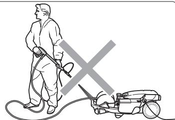
Do not point water and/or sandblast jet at the high pressure cleaner.
