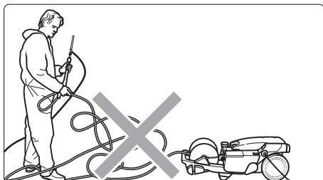
Make sure to prevent kinking and looping of the high pressure hose. Do not pull high pressure hose over sharp edges!
