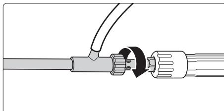
1. Connect high pressure cleaner as with normal cleaning. Connect sandblast injector to gun.
