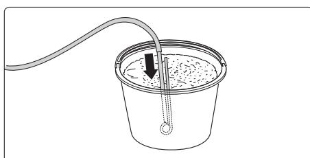
2. Insert suction lance into the sandblasting material container.
