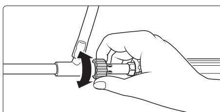
4. The black nut serves to adjust the sand volume. **The blasting material needs to be absolutely dry.**
