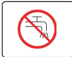
DO NOT FEED WITH DRINKING WATER. USE AN EN 12729 TYPE BA SYSTEM SEPARATOR.
