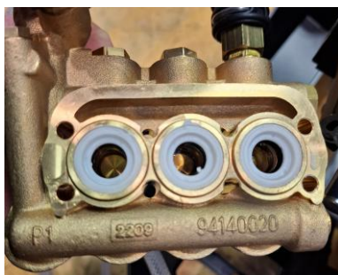
Remove the pump gasket kit using the dedicated puller
