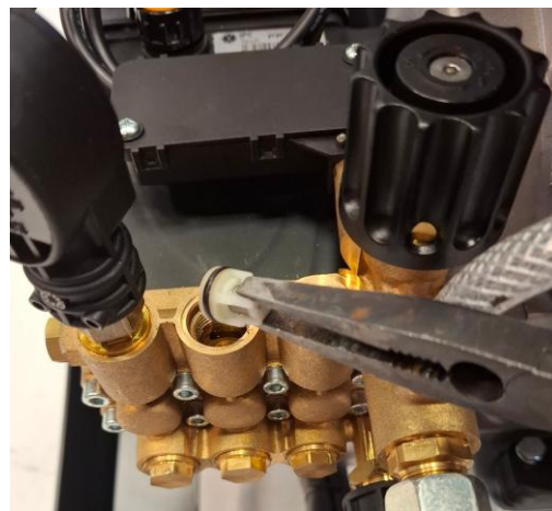
Strip out the valves.
