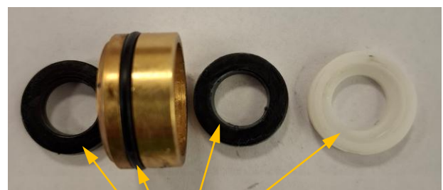
Gaskets that may wear and tear.
