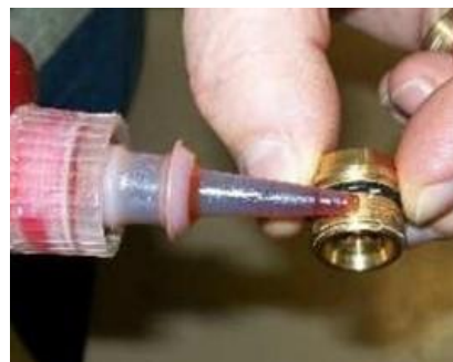
Reassemble the caps using sealing glue type Loctite 542.
