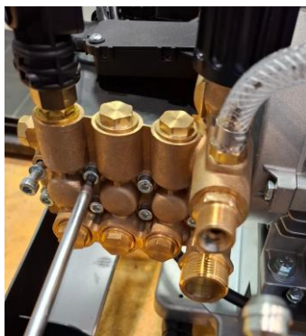
Unscrew the screws that hold the pump head
