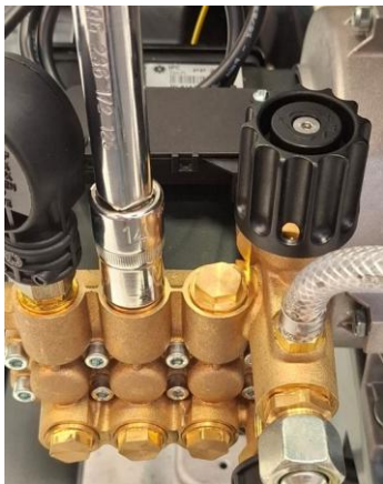
Unscrew the inlet and outlet valve caps
