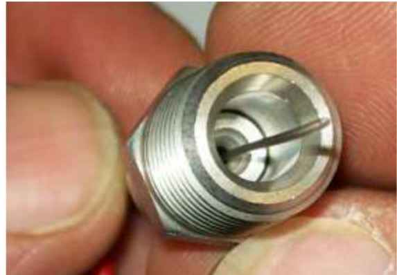
Replacement and cleaning of the high pressure nozzle
