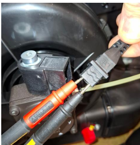
Check the voltage to the fuel solenoid
